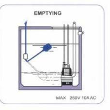
Use wires: "Black" and "Brown" With these contacts the regulator Closes when up Opens when down
