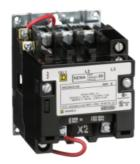
NEMA Contactor, Type S, nonreversing, Size 00, 9A, 3 HP at 575 VAC, 3 phase, up to 100 kA, 3 pole, 120 VAC coil, open
