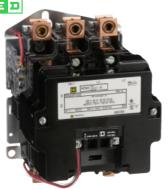
NEMA Contactor, Type S, nonreversing, Size 4, 135A, 100 HP at 575 VAC, 3 phase, up to 100 kA, 3 pole, 120 VAC coil, open
