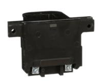
NEMA Motor Starter, Type S, replacement coil, 220/240VAC 50/60Hz, 2 or 3 pole, NEMA Size 2 starters, 8903SP lighting
