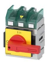
SENTRON, Molded case switch 3LD5 UL, Emergency switching-off, 3-pole, certified according to UL489 UL60947-4-1 and IEC60947-3, UL: 150A, SCCR 50kA at 480VAC, Operating power at 480VAC 3-phase: 100hp, IEC: 160A, Operating power at AC-23A at 400V: 75kW, floor mounting with direct handle, red/yellow, incl. terminal covers for the infeed side
