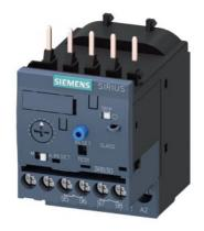
Overload relay 0.1...0.4 A Electronic For motor protection Size S00, Class 10E Contactor mounting Main circuit: Screw Auxiliary circuit: Screw Manual-Automatic-Reset
