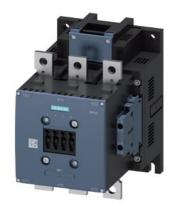
power contactor, AC-3 265 A, 132 kW / 400 V AC (50-60 Hz) / DC operation 23-26 V AC/DC auxiliary contacts 2 NO + 2 NC 3-pole, frame size S10 busbar connections drive: conventional screw terminal
