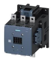
power contactor, AC-3 500 A, 250 kW / 400 V AC (50-60 Hz) / DC 23-26 V AC/DC auxiliary contacts 2 NO + 2 NC 3-pole, frame size S12 busbar connections drive: conventional screw terminal
