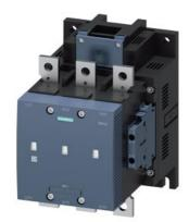
vacuum contactor, AC-3 300 A, 160 kW / 400 V, AC (50-60 Hz) / DC operation 220-240 V AC/DC auxiliary contacts 2 NO + 2 NC 3-pole, frame size S10 busbar connections drive: conventional
