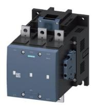
vacuum contactor, AC-3 400 A, 200 kW / 400 V AC (50-60 Hz) / DC operation 220-240 V AC/DC auxiliary contacts 2 NO + 2 NC 3-pole, frame size S12 busbar connections drive: conventional
