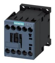
Power contactor, AC-3 9 A, 4 kW / 400 V 1 NC, 220 V AC, 50 / 60 Hz 3-pole, Size S00 screw terminal
