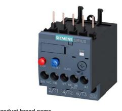
Overload relay 0.18...0.25 A Thermal For motor protection Size S00, Class 10 Contactor mounting Main circuit: Screw Auxiliary circuit: Screw Manual-Automatic-Reset
