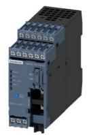
Basic unit SIMOCODE pro V PN GP Ethernet/PROFINET IO, PN system redundancy, OPC UA server, Web server, transmission rate 100 Mbps, 1 x bus connection via RJ45, 4 I/3 Q freely parameterizable, Us: 110...240 V AC/DC, input for thermistor connection Monostable relay outputs, expandable by 1 extension module(DM, TM, EM)
