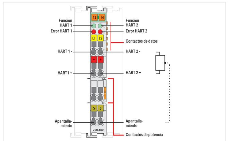
This analog input module powers field-side signal conditioners and transmits electrically isolated analog signals to the bus system. The 24 V field supply is derived from the module's power jumper contacts. The shield directly connects to the DIN-rail. At approximately 25 mA, overload protection switches the measurement input to a high-resistance state. Once normal operating conditions resume, the measurement input will automatically switch back. This module powers 2-wire signal conditioners.
