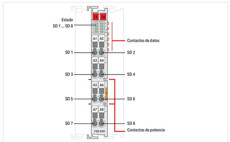
This digital output module features eight channels in a width of just 12 mm (0.47 inch).
