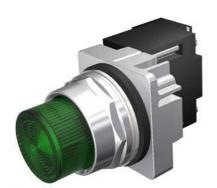
30mm Command/52, Chrome Finish Heavy Duty,Watertight/Oiltight Complete Metal Unit Illuminated Indicator Light Full Voltage type, 120V AC/DC Incandescent Lamp, BA9s Plastic Lens, Green UL Listed, CSA Certified NEMA 1,3,3R,4,4X,12,13 & Automotive Standards
