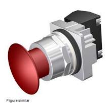
30mm Command/52, Chrome Finish Heavy Duty,Watertight/Oiltight Complete Metal Unit Push-Pull Operator Non-Illuminated Mushroom Head Cap Small 1.73" (44 mm) Metal, Anodized Red 2 Position Maintained, Pull-to-Release with 1 N.O. - 1 N.C. Heavy Duty Contacts, A600/P600 UL Listed, CSA Certified NEMA 1,3,3R,4,4X,12,13 & Automotive Standards
