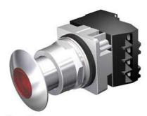
30mm Command/52, Chrome Finish Heavy Duty,Watertight/Oiltight Complete Metal Unit Illuminated Push-Pull Operator Full Voltage, 120V AC/DC Incandescent Lamp Mushroom Head Cap Small 1 3/4" (44.5 mm) Metal, Chrome with Red Lens 2 Position Maintained, Pull-to-Release with 1 N.O. - 1 N.C. Heavy Duty Contacts, A600/P600 UL Listed, CSA Certified NEMA 1,3,3R,4,4X,12,13 & Automotive Standards
