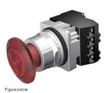
30mm Command/52, Chrome Finish Heavy Duty,Watertight/Oiltight Complete Metal Unit Illuminated Twist-to-Release Full Voltage, 120V AC/DC Incandescent Lamp Mushroom Head Cap Small 1.79" (45 mm) Plastic Cap, Red 2 Position Maintained, Twist-to-Release with 1 N.O. - 1 N.C. Heavy Duty Contacts, A600/P600 UL Listed, CSA Certified NEMA 1,3,3R,4,4X,12,13 & Automotive Standards
