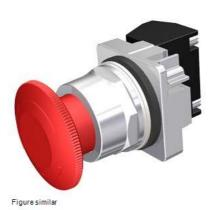
30mm Command/52, Chrome Finish Heavy Duty,Watertight/Oiltight Complete Metal Unit Twist-to-Release Operator Non-Illuminated Mushroom Head Cap Small 1.79" (45 mm) Plastic Cap, Red 2 Position Maintained, Twist-to-Release with 1 N.O. - 1 N.C. Heavy Duty Contacts, A600/P600 UL Listed, CSA Certified NEMA 1,3,3R,4,4X,12,13 & Automotive Standards
