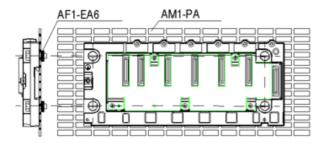
Fasten the rack with four M4, M5, M6 or UNC #6 screws.
