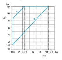
(y) (x) 1: 2: Rising pressure Falling pressure Maximum differential Minimum differential
