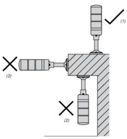
Choose a flat surface with enough strength and with little vibration for installation. Mount this product according to the figure to maintain IP characters of the fig
